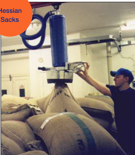
Vacuum Lifter - with spike gripper feature
