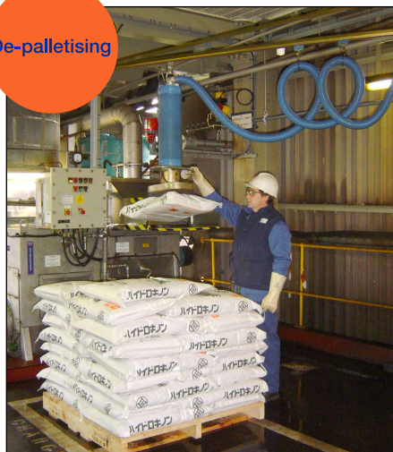
Vacuum Lifter - lifting 25kg sacks
