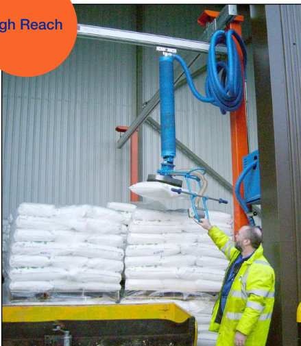
Vacuum Lifter - with flexible extended handle feature for high reach
