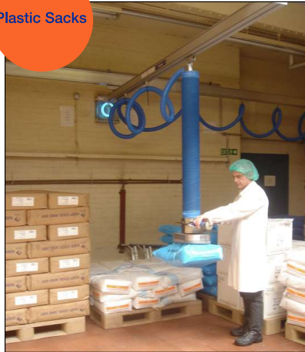
Vacuum Lifter - lifting plastic sacks
