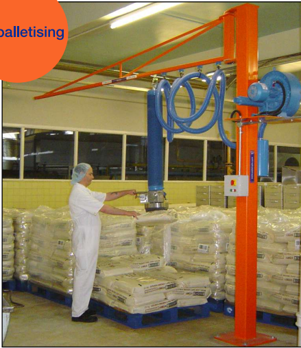
Vacuum Lifter - lifting 25kg sacks
